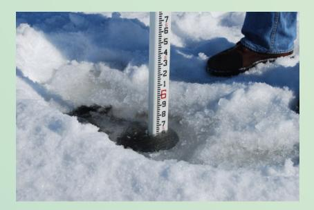
Simply use an ice auger to drill a hole and insert a measuring pole or rod into the hole to get the total depth. If distance from water surface to top of sediment is less than 3 feet, refer to a professional for advice on possible sediment removal. A reference to as-built surveys and design water levels is necessary. You may have less than 3 feet if water levels are low, so record water from the depth gauge levels at the same time. (See page 2.)
